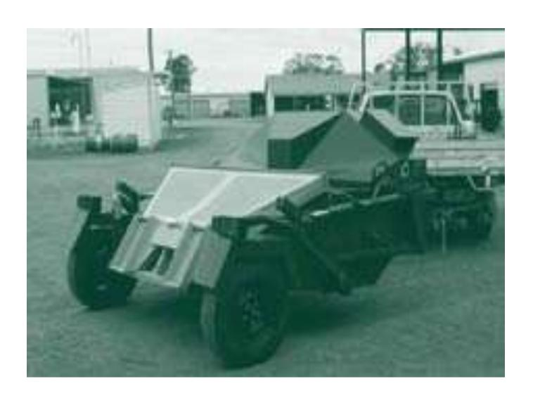
Picture 3. The DLWC 'Grasshopper' is light weight (500–750 kg), has adjustable brushes and harvest height. The 'off-set' working position facilitates harvesting ripe seed that has not been disturbed by the towing vehicle. (Photograph C. Huxtable)
