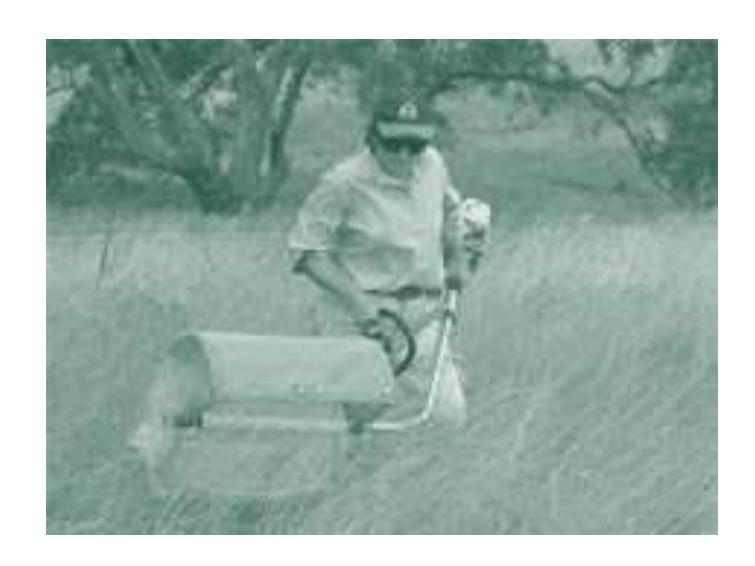
Picture 5. A reel and brush harvester which gathers culms with inflorescences over the top of a rotating brush to deposit the seed in a seed hopper. Designed and built by J. Stafford, Vegetation Management Services, Main Rd, Lenswood. SA 5240 (Photograph R. Whalley)
